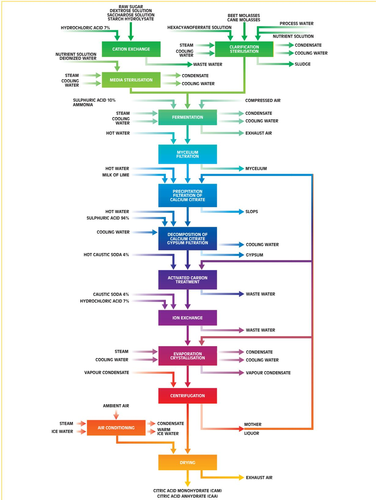
Figure 3: Block diagram - Vogelbusch process for citric acid production
